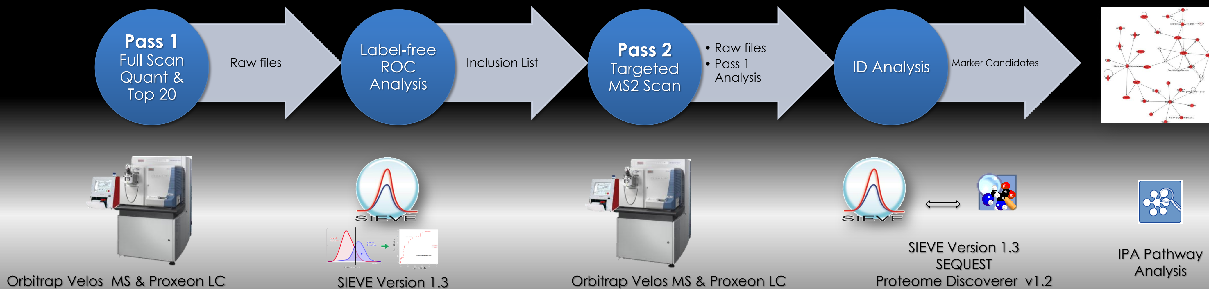
FIGURE 2. BRIMS Two-Pass workflow (left to right): A) High-quality full scan acquisition with five technical replicates on Thermo Velos Orbitrap and Proxeon nano LC including a top-20 data dependent method, B) Label-free processing with SIEVE v1.3 including PerfectPair analysis to produce an inclusion list, C) Targeted acquisition with high quality fragmentation scans, D) ID analysis with SEQUEST, Proteome Discoverer, and SIEVE.
